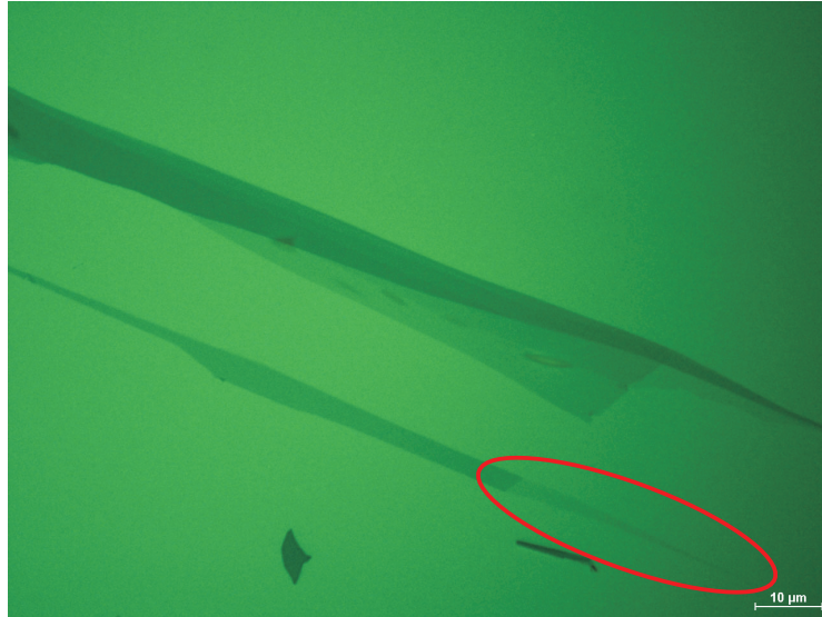
Figure 3.1: An optical image of monolayer graphene (encircled area) on top of Si/SiO 2 .
