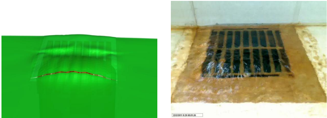
Figure 5.19 – Visual comparison of simulated and observed water surface features, surcharged conditions, flow rate = 13.89 l/s
