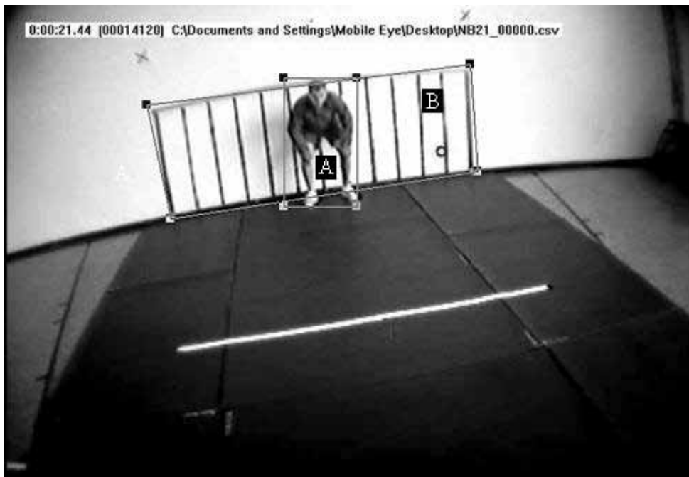
Figure 5. A screen grab from the GazeTracker software environment showing the experimental setup and the two “LookZones” (areas of interest): the goalkeeper (A) and the goal area (B). The circular cursor, to the goalkeeper's left, represents the participant's point of gaze.
