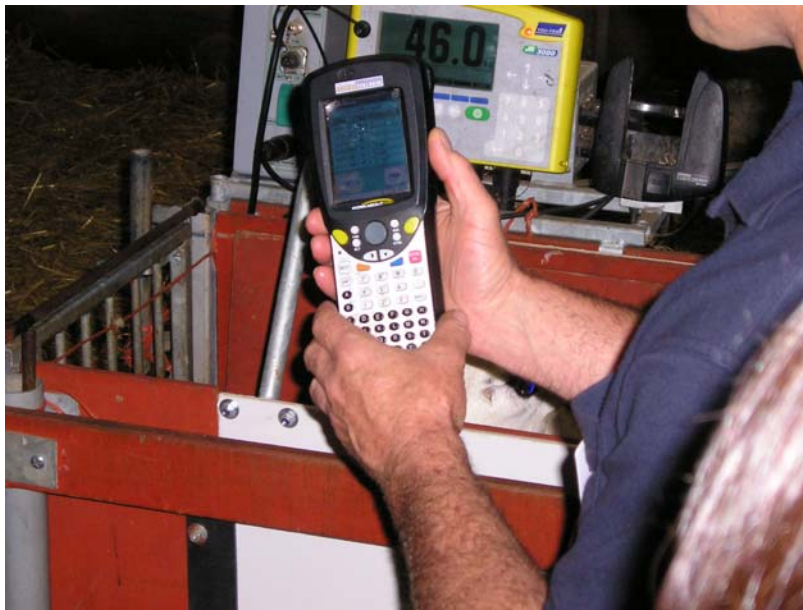
Figure 6.4: Handheld EID Scanner being used to read the tags of individual sheep. As they are run through a race their weight is being measured and automatically recorded. The information is then sent electronically to the mainframe computer, where records are held. (Authors own image)
