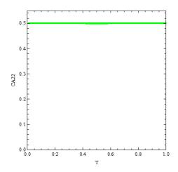
Figure 8.3: With  $\alpha = dL = 0$ , AUTO is used to output the value of  $C_{22}^A$  as T is increased from 0 to 1. At these values of  $\alpha$  and  $dL^*/\lambda C_{22}^A$  is fixed at 0.5 allowing us to simplify the equations further.
