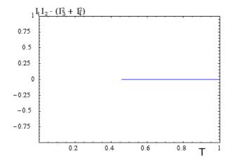
Figure 7.15: In contrast to Figure 7.14 this figure shows how  $I_1I_2 - (I_3^2 + I_4^2)$  remains zero as the Hopf bifurcation is continued. This is indeed a correct bifurcation and is verified by DsTool and Matlab.
