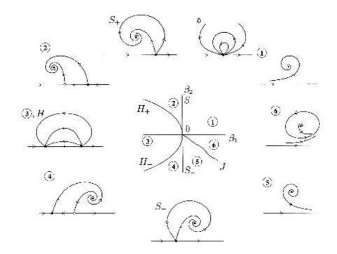
Figure 7.7: Unfolding of the Saddle-node Hopf Bifurcation as shown in [23, p343].
