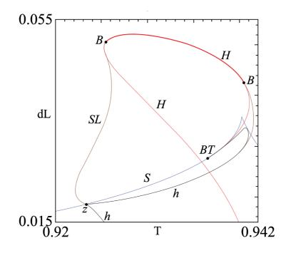
Figure 7.4: A region of the lasers parameter space, for Figure (6.5) with  $\alpha = 0$ , showing three types of codimension-2 points; Bogdanov-Takens (BT), Bautin (B), and a non-central Saddle-node Homoclinic point with additional non-centrality (Z). Also indicated here is the nature of the Hopf curve; the supercritical region is shown in bold red, while the subcritical part of the curve is in fine red.
