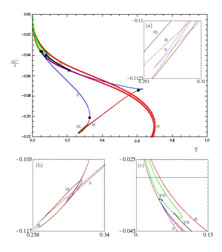
Figure 6.6: Bifurcation diagram for  $\alpha = 1$ : steady and periodic solutions. Homoclinic bifurcations, h, joining with the two saddle node Hopf points can be seen in black. Note the presence of torus bifurcations (T) from SH to PD at a codimension two interaction. Note the presence of torus bifurcations, T, from SH to PD lines at a codimension two interaction.
