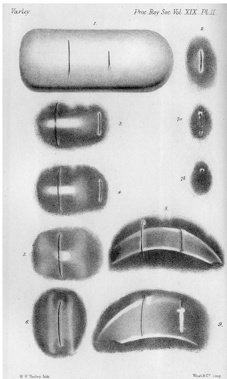
Figure 3. Photography of electrical discharge in a Geissler tube. This sequence of images represents the changes in the visual and/or photographic appearance of electrical discharge as the resistance in the circuit is changed. In images 1 to 5 the eye and photographic plate tell approximately the same tale. '1.' shows the Geissler tube with its circular electrodes in plan view; '2.' shows that with a high resistance in the circuit there was luminosity around the right-hand or positive pole only; '3.' and '4.' show that with lower resistance luminosity was seen projecting from the positive to the negative pole which was itself beginning to emit light; and '5.' shows that at lower resistance still, the luminosity around the positive pole was extinguished. Image '6.', however, shows that according to the photographic plate, when the resistance was removed altogether the positive pole was surrounded by a luminous white hour-glass shape. To the eye, however, this pole was shrouded in a 'bright blue envelope'. Reproduced by permission of the President and Fellows of the Royal Society of London.
