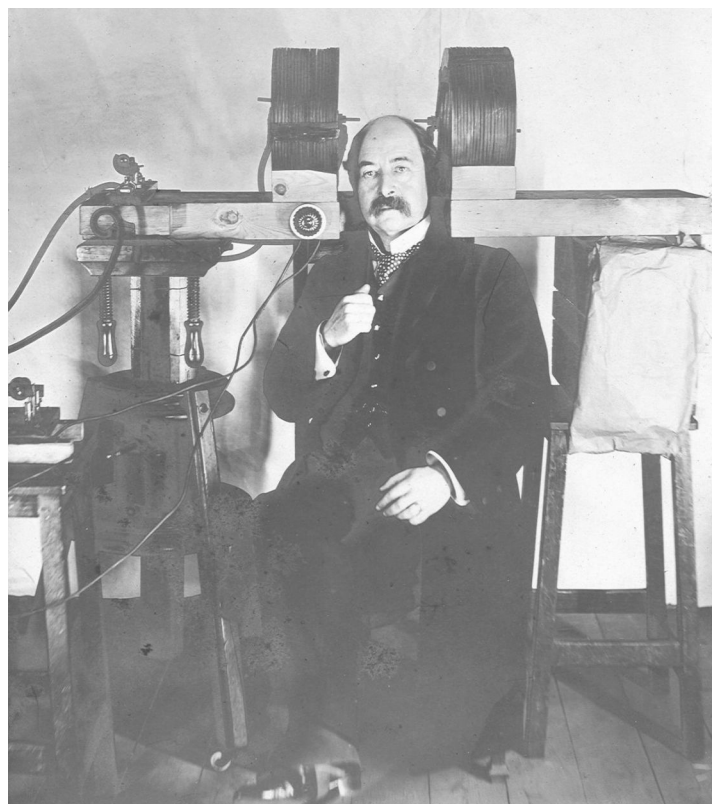
Figure 4. Silvanus Thompson FRS testing the physiological effect of a large alternating magnetic field. Photograph accompanies letter, J. Crichton-Browne to S. P. Thompson, 4 Apr. 1910, Thompson Papers, Imperial College London Archives, 63a. Reproduced by permission of Imperial College London Archives.
