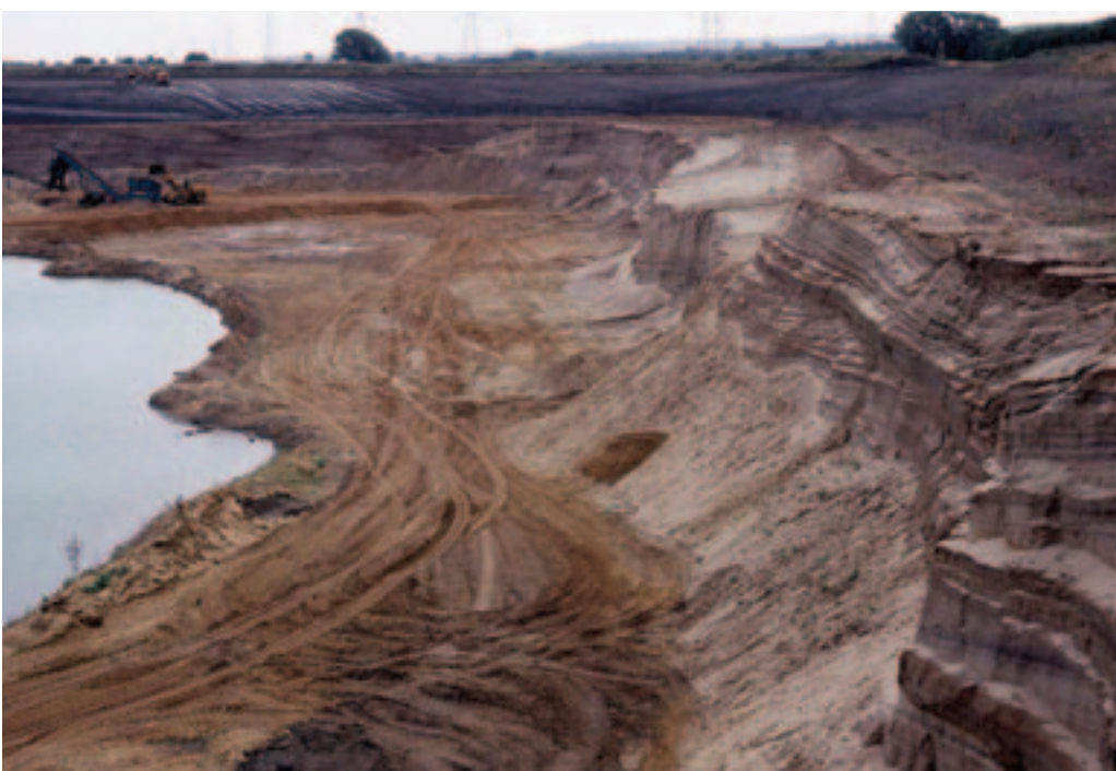
Cross-bedding in Lower Cretaceous, Lower Greensand overlain by Gault Clay. Pratts Quarry, Leighton Buzzard, Bedfordshire.
