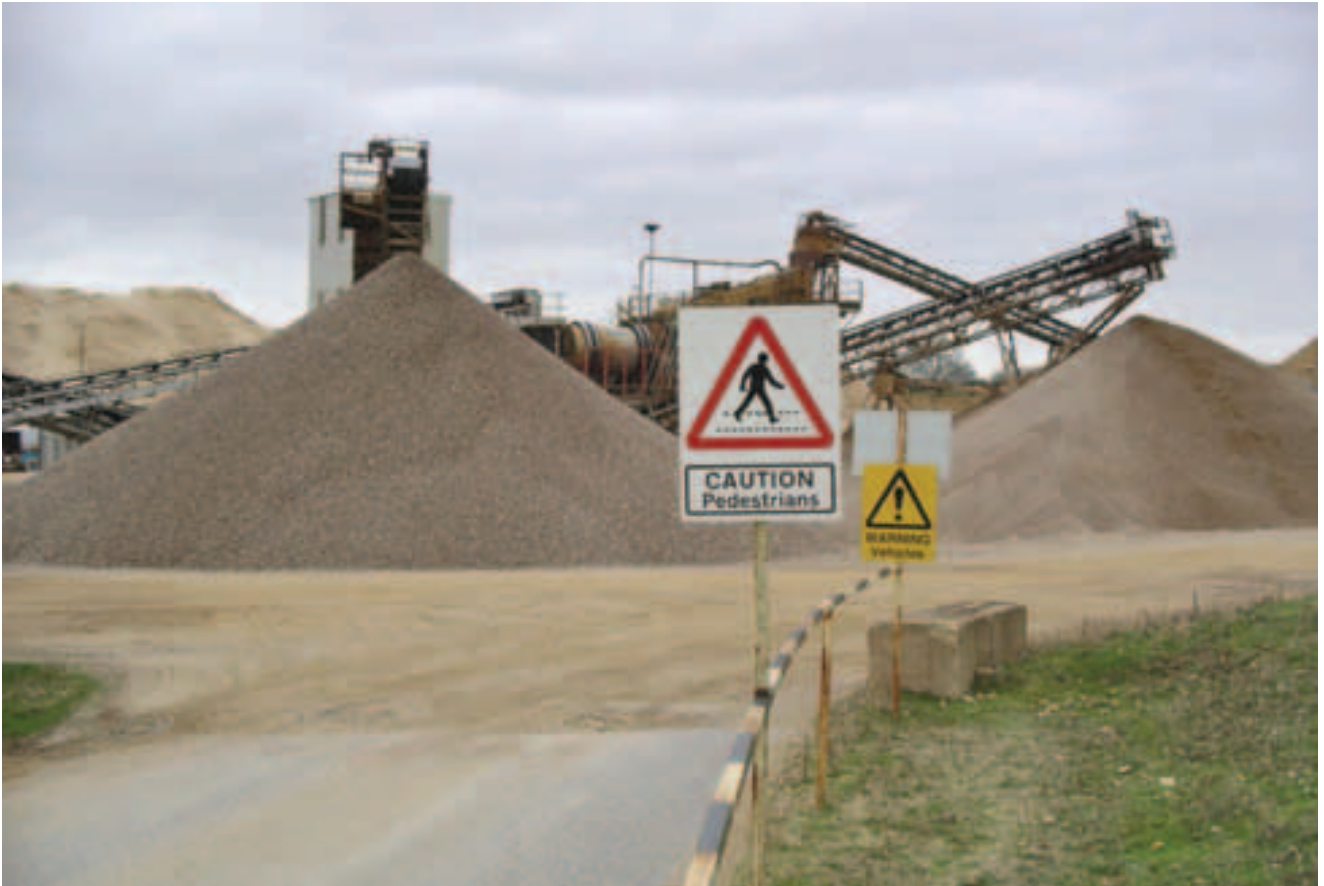
The processing plant area of a quarry presents hazards to the geological visitor who usually has to pass through it on the way to the quarry faces. Transport by vehicle through the processing plant or via a designated and separate pedestrian route may be required.
