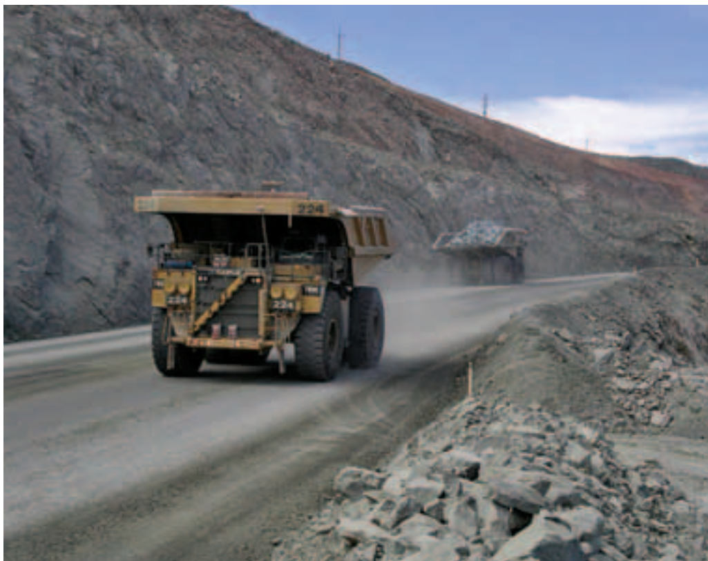
Large trucks, each capable of hauling 240 tonnes of rock. Access by pedestrians to the haulroads in this open pit is extremely dangerous and forbidden as there is a haulage truck passing about every minute during the working day. The photograph was taken at a refuge part way up the haulage ramp. This enables visitors to see the geology. Superpit gold mine, Kalgoorlie, Western Australia.
