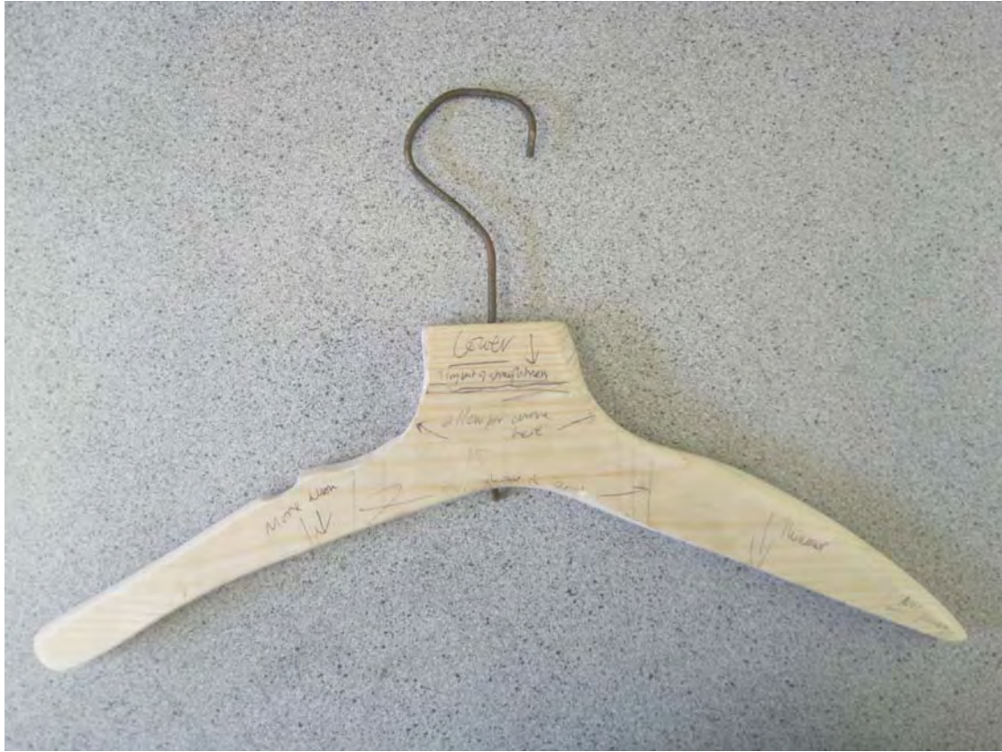
Figure 2: Test coat hanger with comments on shape. Coat hanger project (2009).
