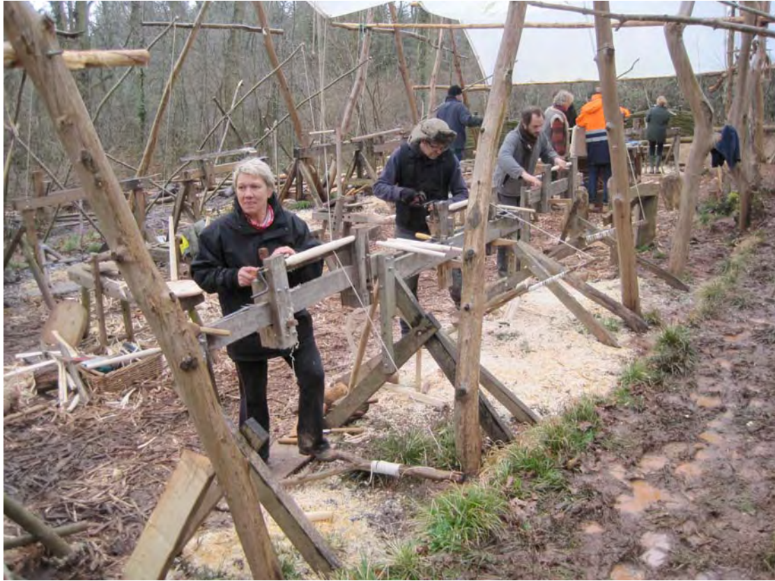
Figure 18: Suzanne Barnes, Rory Dodd and Gareth Neal using manually powered pole lathes. Part of Bodging Milano (2010).
