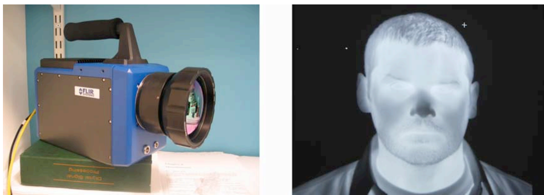
Fig.12: thermal image camera
