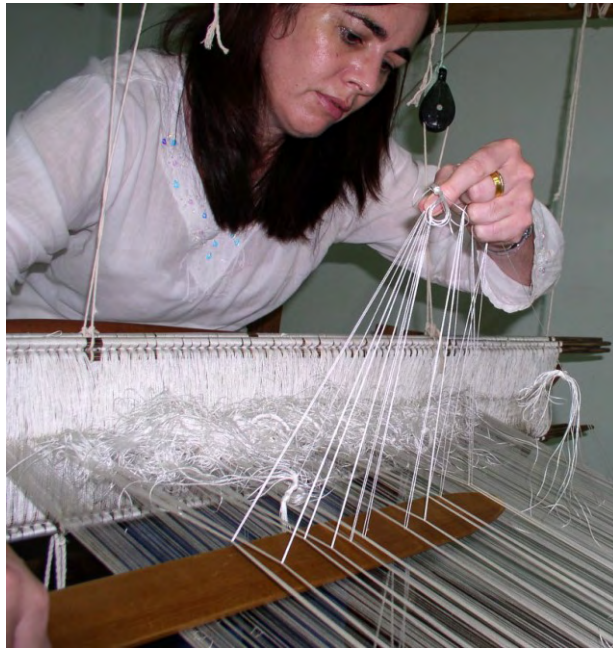
Figure 5.28. Top, the author lifting butang and inserting shed stick which often snags the fine warp yarns. Lower (x2), turning the shed stick on its side lifts the warp yarns and places them under tension which also causes breakages.
