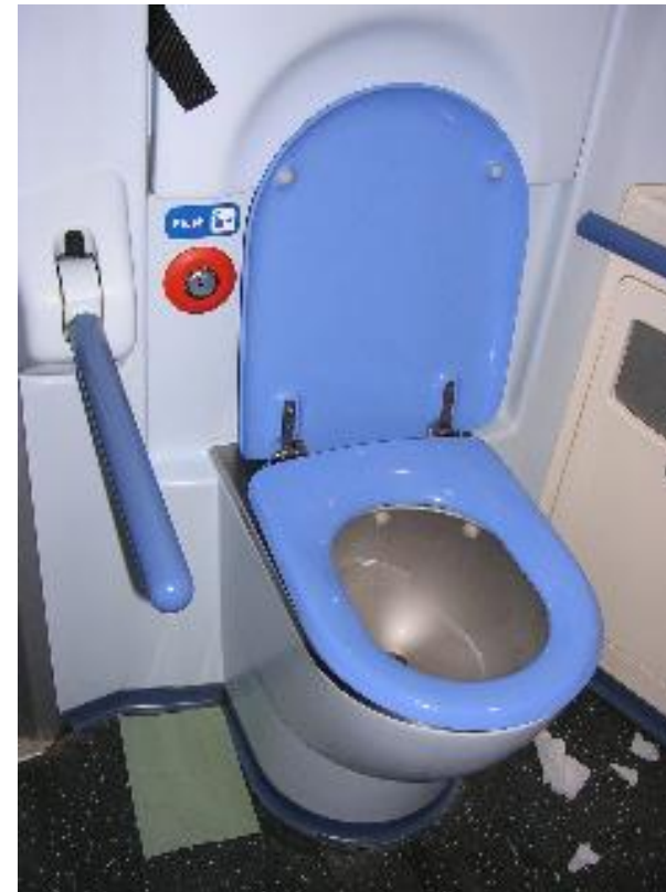
Sensor and automatic flushes can be disconcerting for users of accessible facilities. (Bichard 2004) VivaCity 2020
