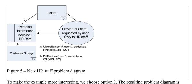
shown in Figure 5. The diagram shows that the user is to supply some sort of credentials along with the request for information. These credentials are passed to an external authentication and authorization engine, which answers yes or no. If the answer is yes, then the machine provides the data; otherwise, the data is refused. The corresponding behavior specification is:
