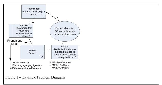
Problems are described using a straightforward graphical notation. Domains are boxes, interfaces are arrows, and phenomena are described by indicated by a label on an interface. Figure 1 shows a problem diagram for a simple alarm system. It has one requirement: sound an alarm for 30 seconds when a person enters the room under protection.
