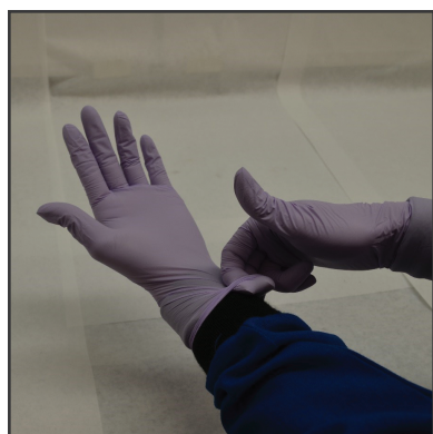
(A) Start by hooking a finger into the outside of the glove.
