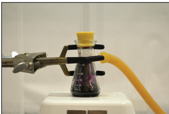
(C) As the temperature rises, more crude material sublimates. Inside the filter flask, the vapor reaches the cold finger. The vapor then crystallizes immediately.
