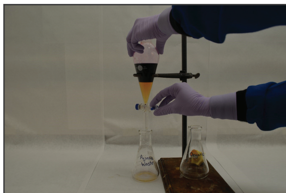
(B) The two phases are separated. The aqueous (or lower phase) is drained into a clean container.
