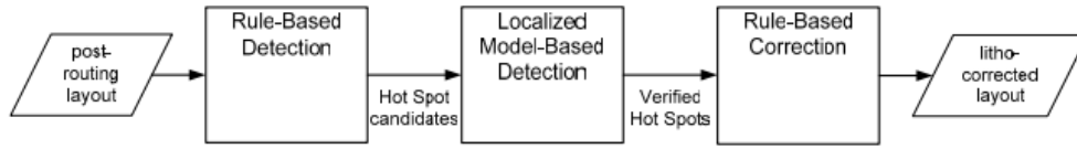
Figure 6.4: Rule-Based Detection identifies hotspot candidates. These candidates are then confirmed or rejected by lithography simulation. Finally, hotspots are fixed by Rule-Based Correction. Figure from [73]
