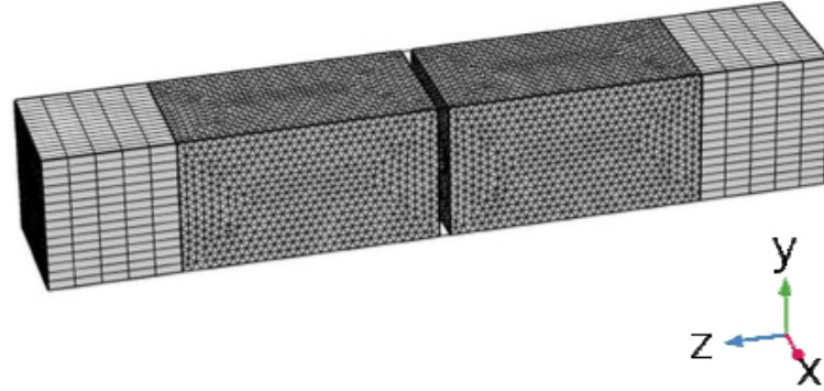
Figure 3.6: Meshing of both devices is defined by a physics controlled mesh with maximum element size equal to \frac{\lambda}{6} . The maximum element size of the IBC boundaries is defined to be less than the skin depth of both materials.
