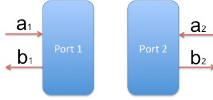
Figure 3.1: The power wave parameters. a_1 is the incident power wave on port 1, b_1 is the reflected power wave on port 1, a_2 is the incident power wave on port 2, b_2 is the reflected power wave on port 2.
