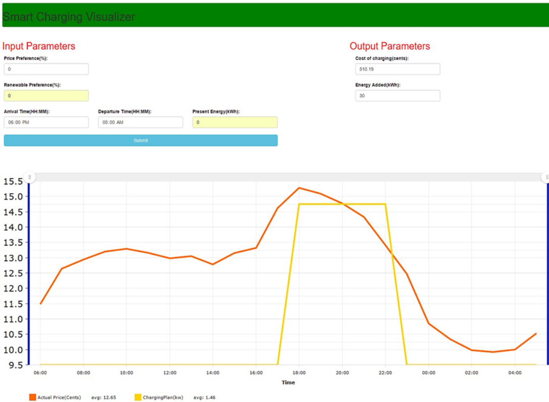
Figure 2.3 Smart charging visualizer depicting normal full – rate charging of EVs
