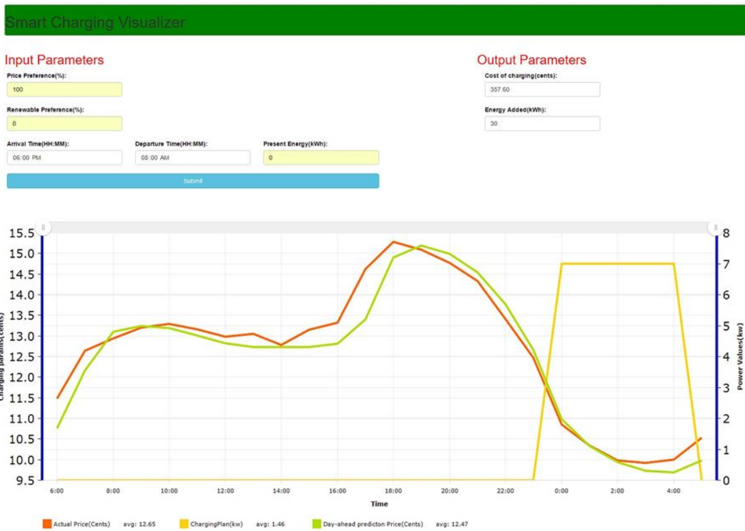
Figure 2.7 EV smart - charging visualizer depicting smart – charging scenario with day ahead predicted grid load information
