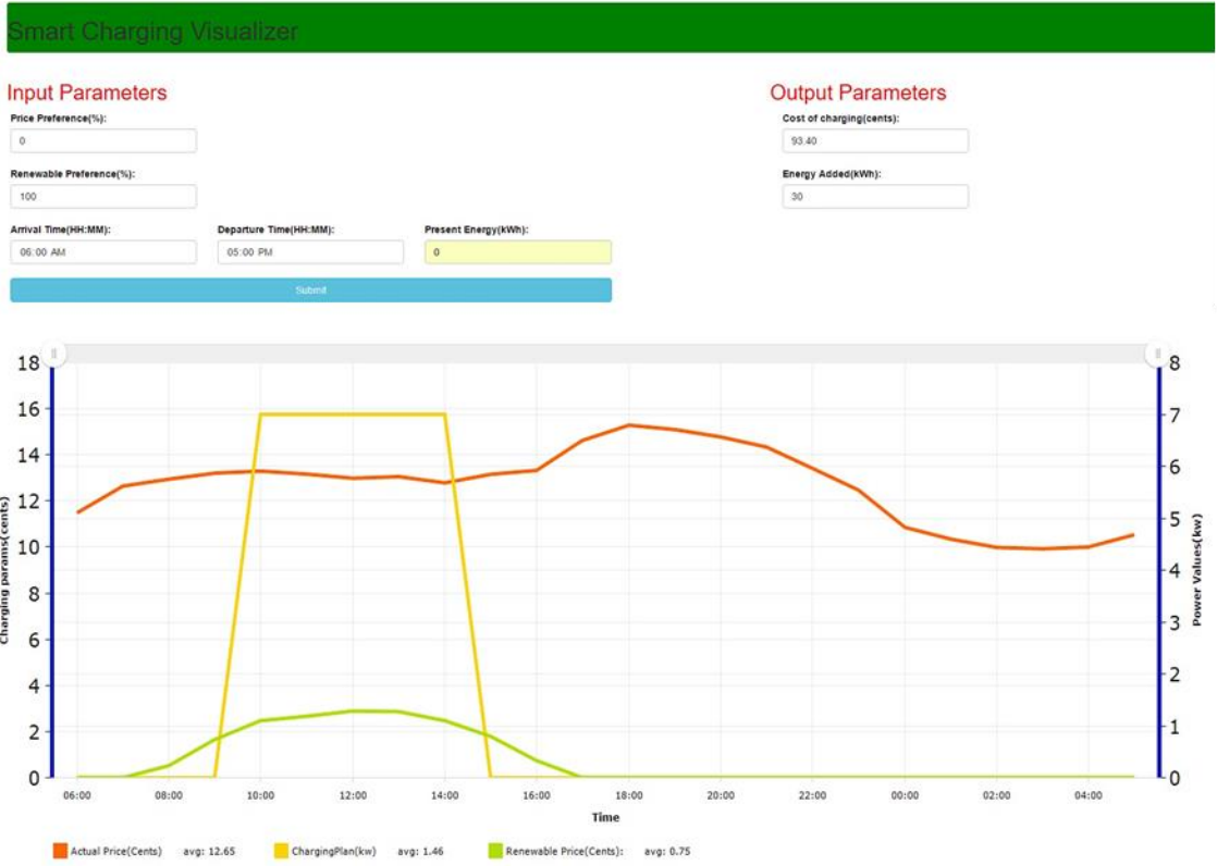
Figure 2.10 EV smart - charging visualizer depicting smart – charging scenario with perfect grid load information and solar energy
