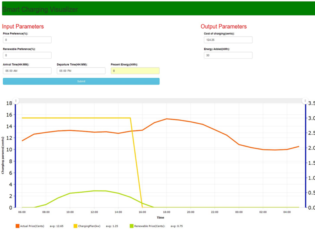
Figure 2.9 Smart charging visualizer depicting half – rate charging of EVs
