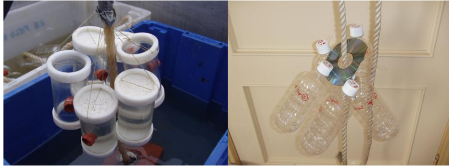
Figure 37 Semi-permeable membrane bottles for Shallow and Deep treatments (left) and sealed bottles for Control, N+, P+ and N+P+ treatments (right)
