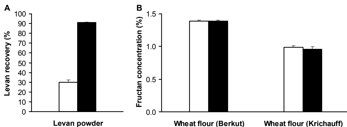
Figure 4 (A) Recovery of pure levan (Sigma L8647) and (B) fructan concentrations of wheat grain (cv. Berkut and cv. Krichauff) measured by the proposed method applying different digesting conditions: (□) 1 unit of inulinase for 30 min and (■) 3 units of inulinase for 90 min. Error bars represent standard errors of the mean of three determinations.
