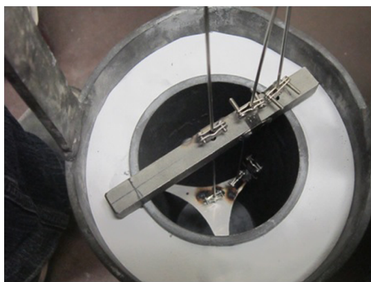
Figure 5. View of the graphite crucible with the Inconel shell and the thermocouple-holding structure before the melting of the synthetic cryolite.
