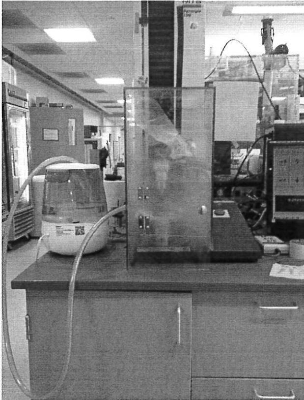
Figure 39. Setup for humidity testing
