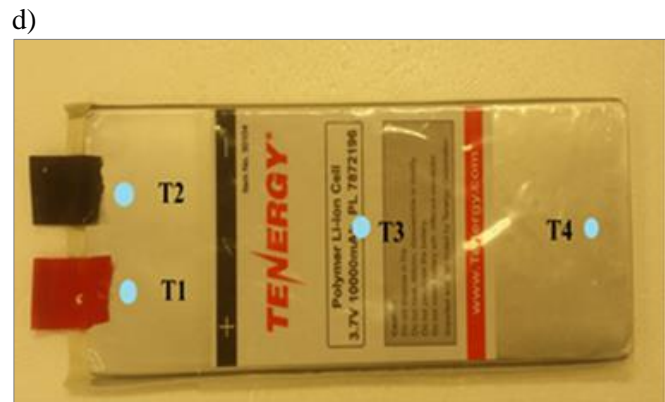
Figure 4.3. Surface temperature profiles at a) 0.1 C-rate, b) 0.5C-rate and c) 0.8C-rate. d) Temperature is measured closed to the positive tab (T1, blue lines), close to the negative tab (T2, orange lines), center (T3, red lines) and at the bottom of the battery (T4, yellow lines).
