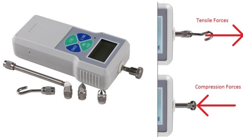
Figure 9. Example of a Dynamometer used in forces measurements (image adapted from www.aliexpress.com/Digital-Dynamometer-Force-Measuring-Instruments )
