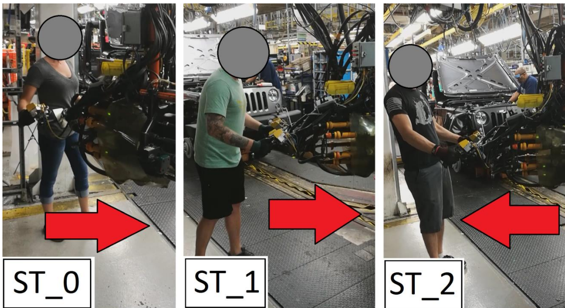
Figure 17. Sub-tasks performed on WS 7 ; the red arrows represent the principal direction of motion of the component in the identified sub-task.
