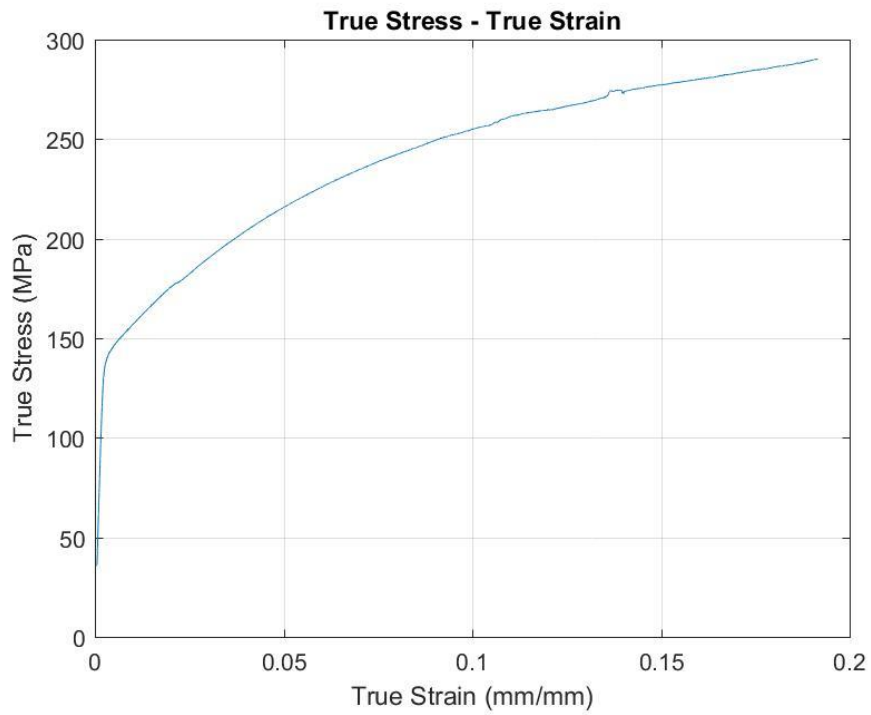
Figure 4-16: True Stress-True Strain curve for Quiet Aluminum® with 6061-T4 skin in the as-received condition. Uniform deformation after the elastic region.
