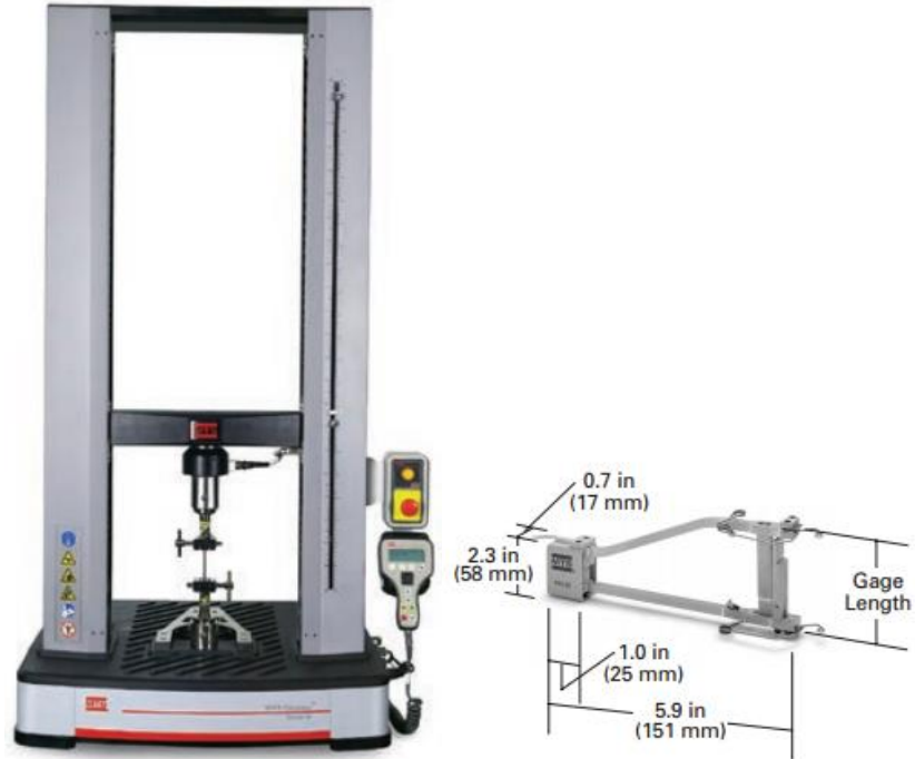
Figure 3-5: MTS Model 43 Universal Tensile Testing Machine and MTS Axial Extensometer 50 mm gauge length [44].
