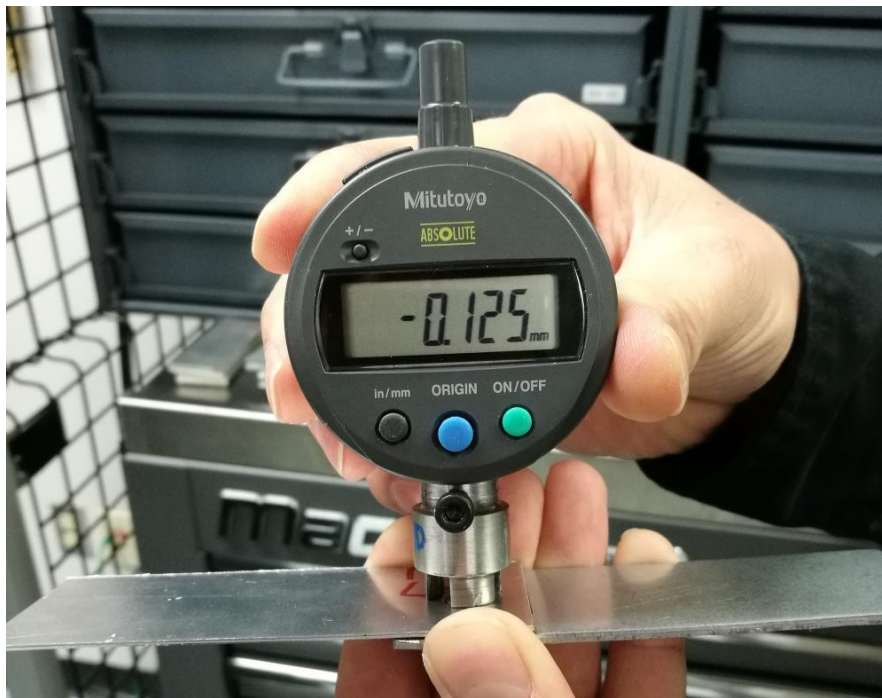
Figure 3-12: Example of the rivet head measurement using connected dial gauge.
