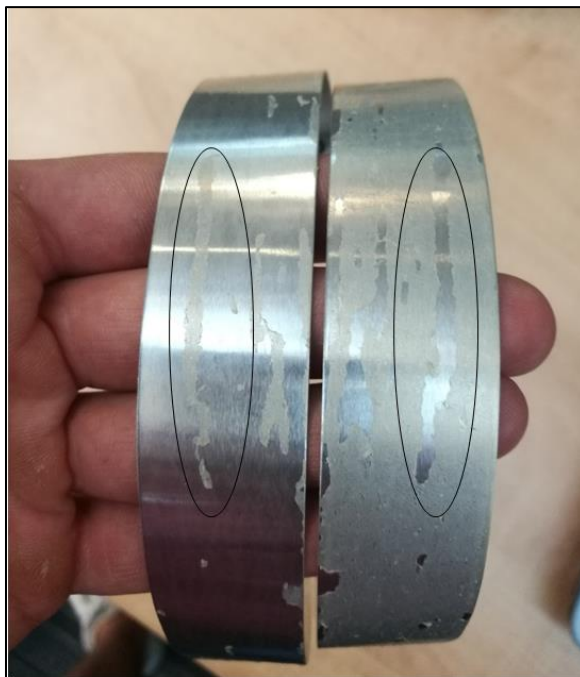
Figure 4-34: Quiet Aluminum® strips with AA5754-O skin after the paint-bake simulation (20 min at 185°C). The image shows the inner surfaces of the sandwich after T-peel test. The specimen presented adhesive failure mode. The black circles are examples of the polymer attached to one surface and the other in a complementary way.
