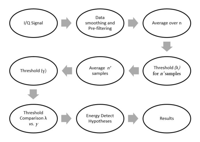
Figure 3.8: Block Diagram of Utilized Sensing Algorithm
