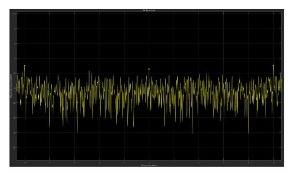
Figure 4.7: Peak detection in ATSC Signal
