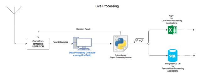
(a) Detected signals pre-processing flowchart
