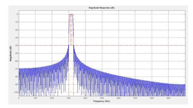
Figure 3.7: Magnitude Response of Band-pass filter
