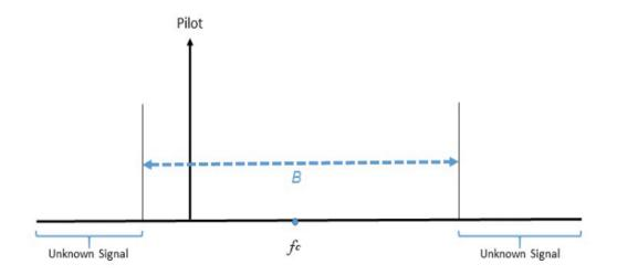
Figure 2.6: Pilot Signal in Spectrum
