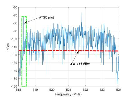
Figure 4.12: Observed pilot-tone for channel 22
