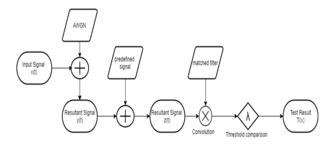
Figure 2.8: Block Diagram of matched filter technique
