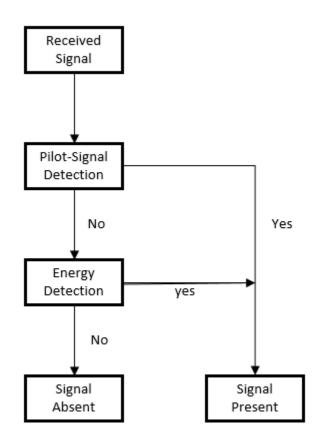
Figure 3.5: Block Diagram of Two step spectrum sensing Technique
