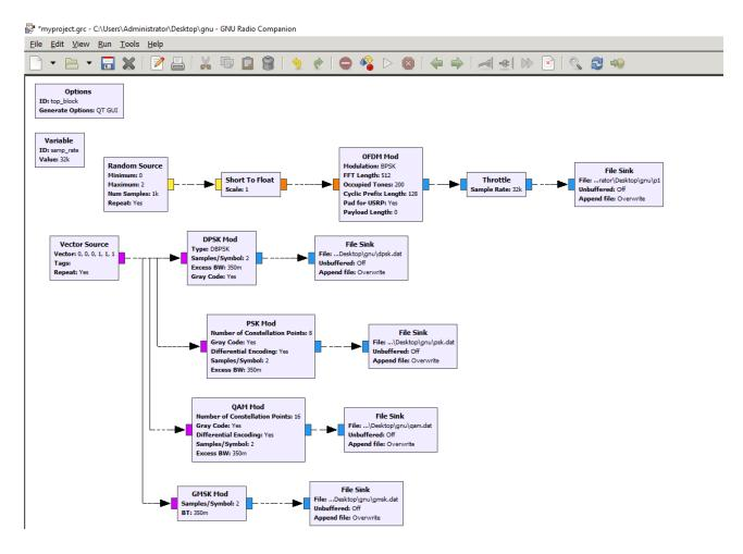
Figure 3.4: GNU Radio Program for data generation
