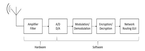
Figure 2.2: A simple Software Defined Radio
