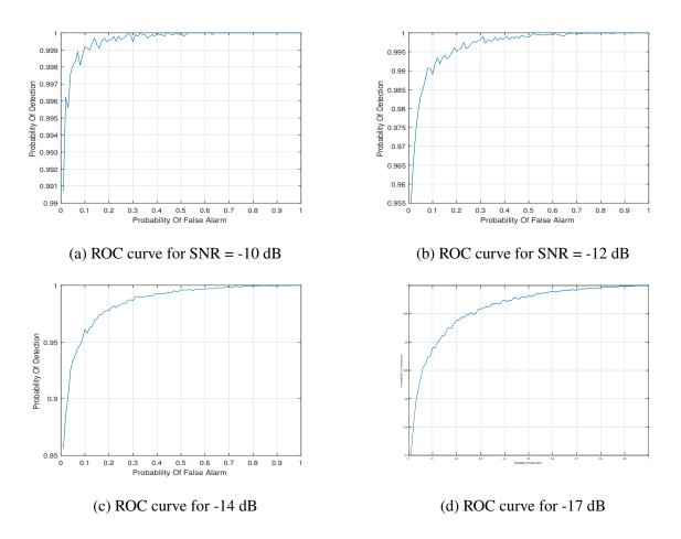
Figure 4.19: ROC plot for probability of detection and probability of false alarm
