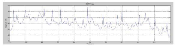
(c) Gaussian Minimum Shift Keying Modulated Signal
