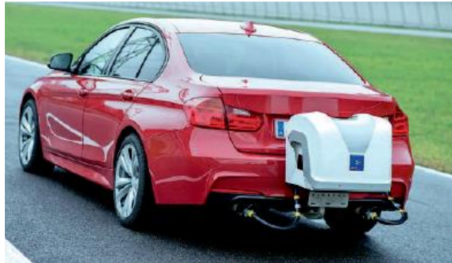
Figure 2.8 The AVL M.O.V.E GAS PEMS is Portable Emission Measurement System (PEMS) [28]
