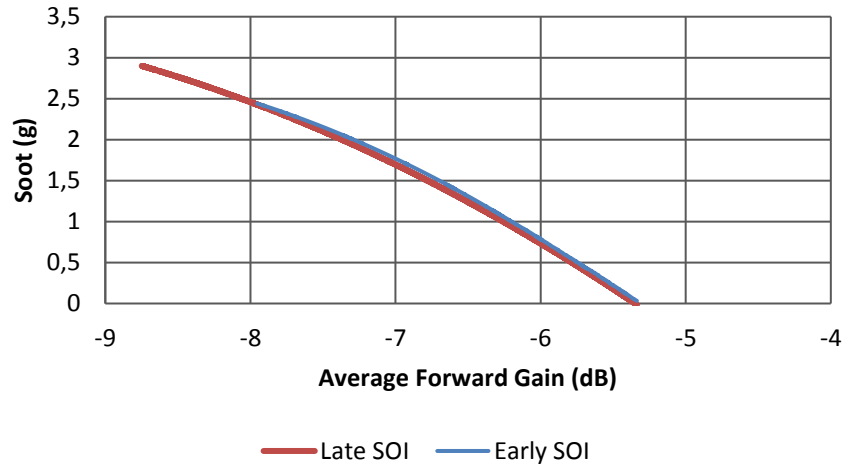
Figure 57: Soot as a function of average forward gain for late SOI and early SOI conditions.
