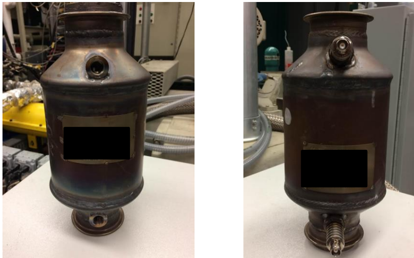
Figure 26: Uncoated (left) and coated (right) filters.
