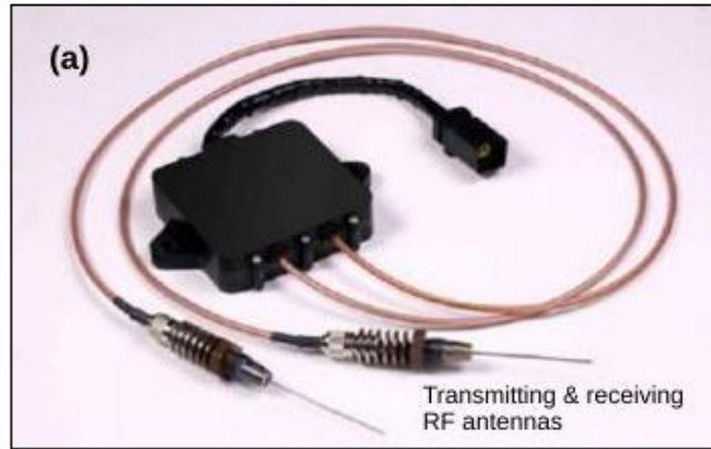
Figure 14: GE Accusolve RF sensor with two antennas [31].
