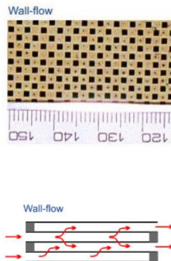
Figure 8: Wall flow substrate: inlet cell pattern (above), flow pattern (below) [24].
