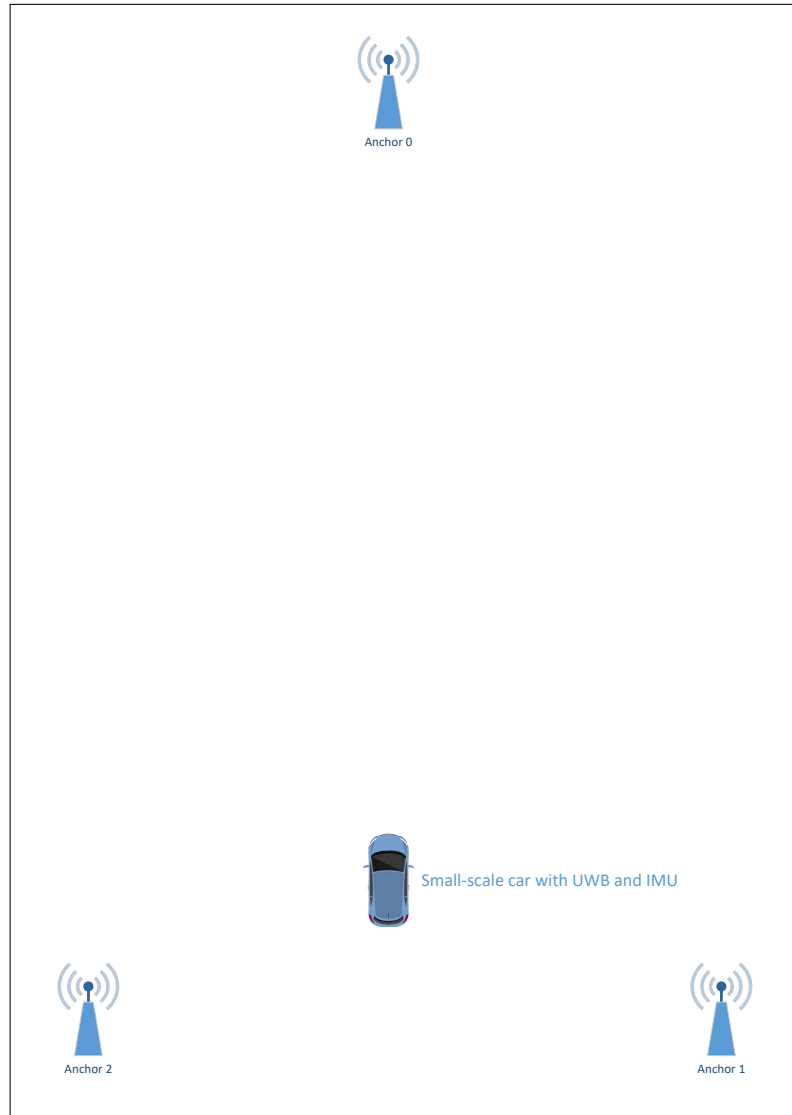
FIGURE 3.4: Experimental setup of experiment in the hallway (not to scale).
