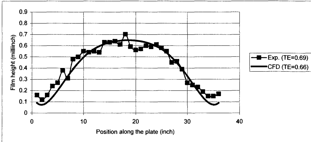
Figure 6.8 Paint Film Thickness Profile and Transfer Efficiency (paint flow rate = 200 cc/min, shaping air flow rate = 250 cc/min)
