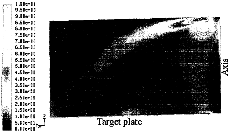
Figure 5.28 Meridian View of Air Velocity Magnitude Contours at 90 kV
