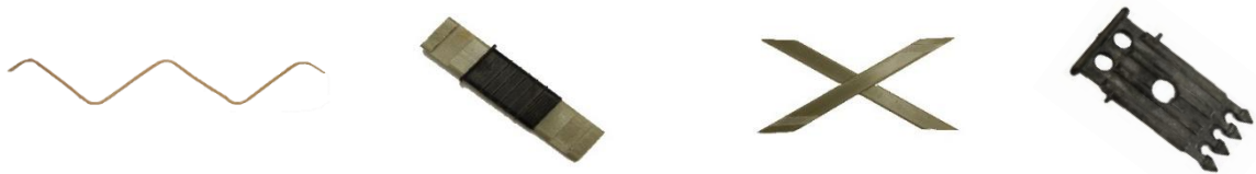
Figure 3-1 Shear Connectors Tested, Left to Right: Connector A, B, C, and D
