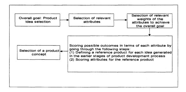
Figure 3.7. Five-step product idea selection process based on AHP
