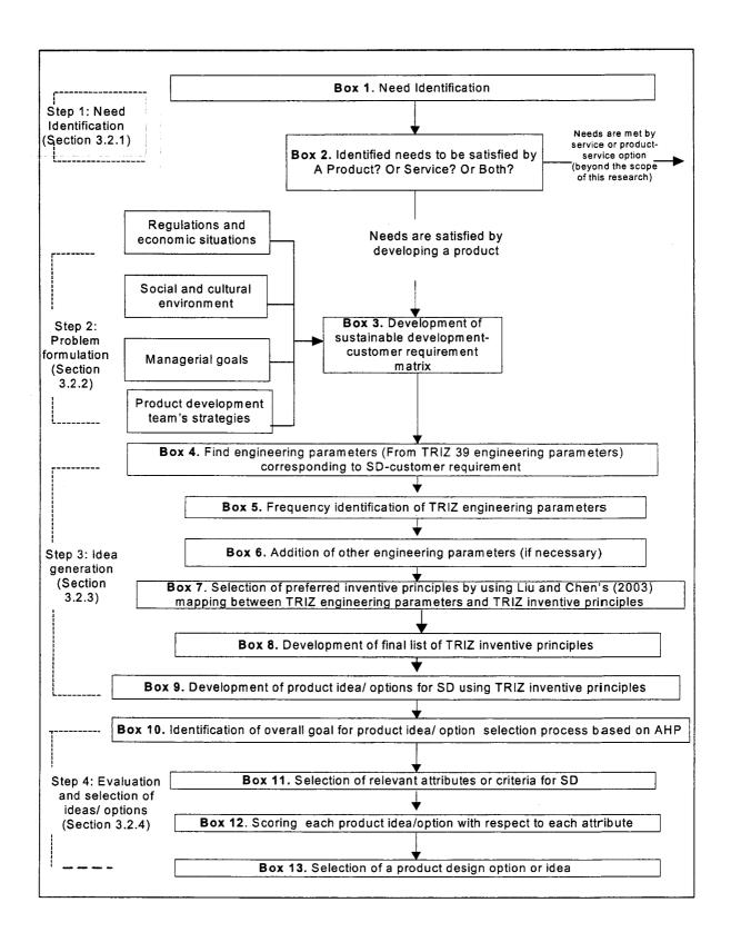
Figure 3.1. Methodology Diagram
