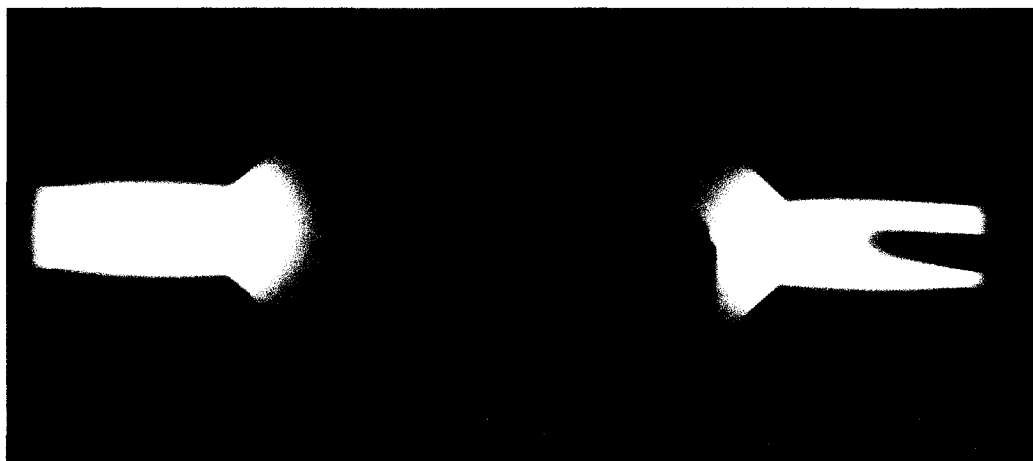
Figure 4.2 Temperature profile for a sample with extension length of 30mm and central zone width of 40mm.
