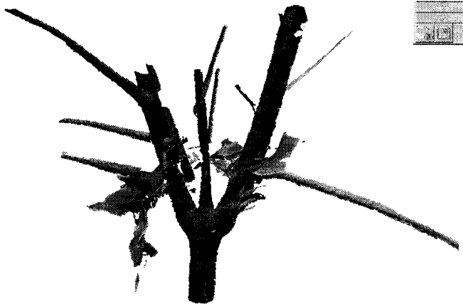
Figure 14: High resolution scan of a section of a Maple tree branch. Minolta Vivid 910, Resolution: 625 dot in 1 inch.
