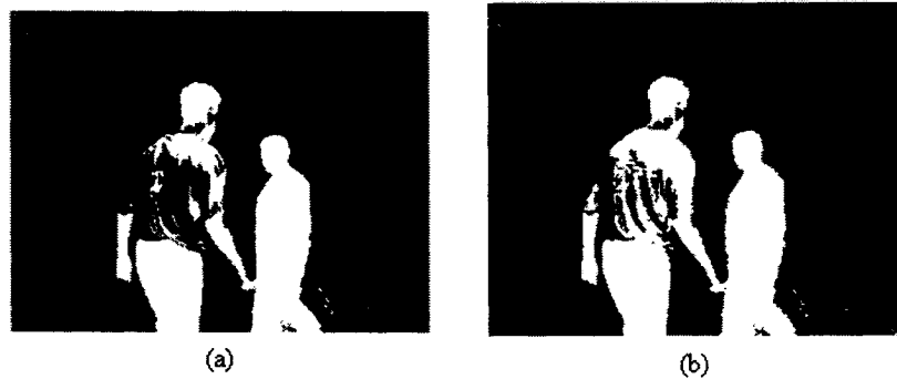
Figure 5.9: Problems in Segmentation: (a)Partially segmented part of shirt,(b)almost detected region after considering chromaticity information
