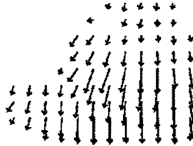
Figure 2.5: An example of optical flow: Moving objects identified using these motion vectors
