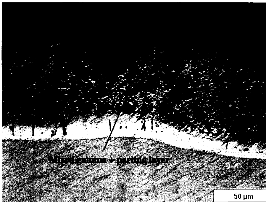
Figure 36: Mixing of the parting and gamma-brass layers in a FIN-12 electrode. The mixed layer had an average thickness of 40 μm and was only evident at the centre of the electrode face.
