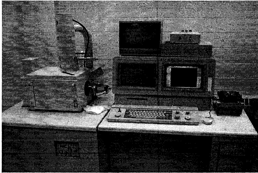
Figure 3.9: Scanning electron microscope (Joel Model JSM-5800LV).
