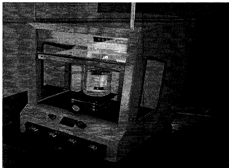
Figure 3.10: Experimental setup for density measurement.
