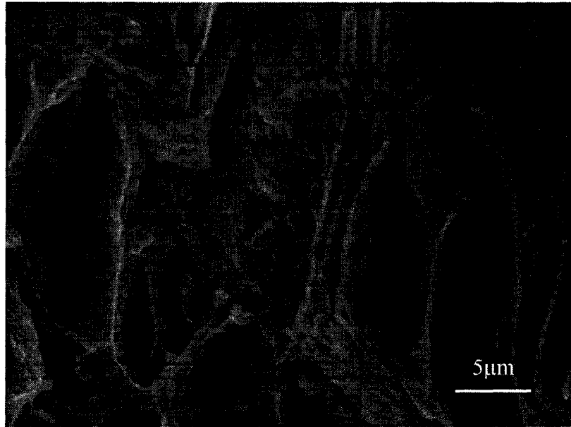
Figure Ap3.7: SEM fractographs of squeeze cast AMC504 under 30 MPa at 150 °C.
