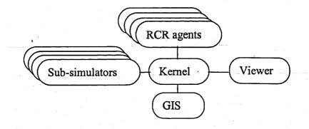
Figure 3-1 Structure of the RCRSS
