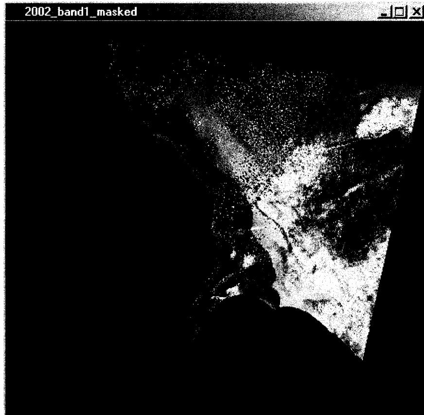
Figure 3.11: 2002 Band 1 Masked Showing Land Values in Black, and DN Values for Offshore Areas
