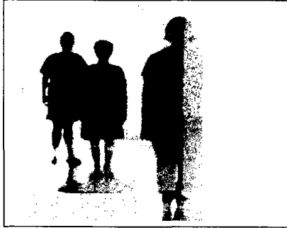
The binarised moving pixels image resulting from the background subtraction operation
