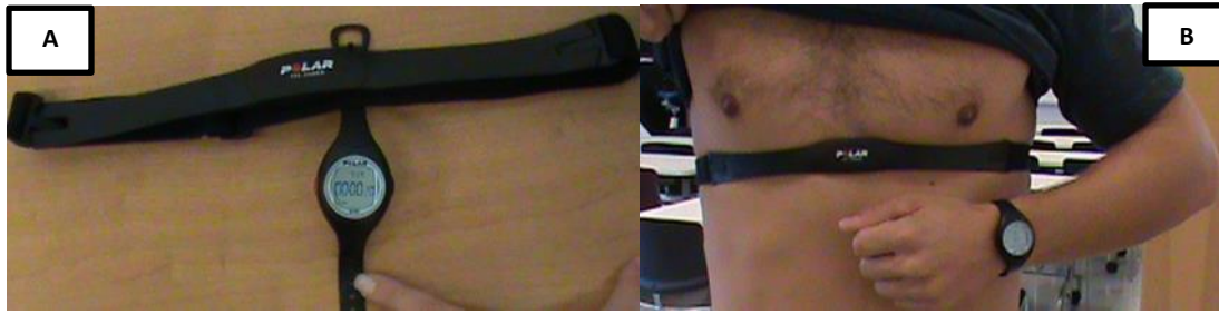
Figure 3: A is the Polar Heart Rate Monitor (Model E40) watch and the corresponding chest strap. B is the proper placement of the Polar Heart Rate Monitor chest strap. The chest strap should rest below the nipples and be centered just below the sternum.
