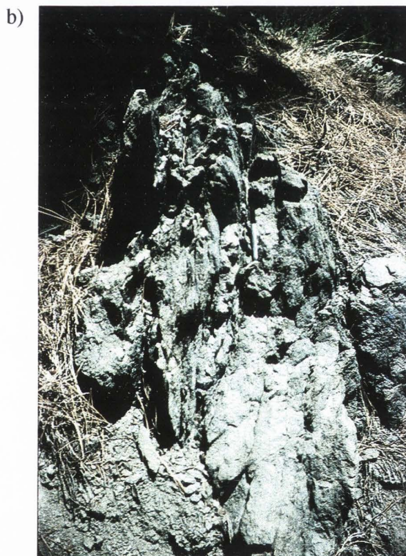
Fig. 9 Rock outcrops north of the fault core at traverse 1. a) Pelona Schist 80 meters north of the Punchbowl fault. The schist is undeformed, with little fracturing along the foliation. b) Exposure 47 meters north of the Punchbowl fault. The schist is more deformed than in the previous photo, with increased fracturing along foliation. c) The schist 30 meters north of the Punchbowl fault is strongly deformed and the schistose foliation is difficult to identify.
