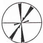
TRAVERSE PT G (Outcrop Fractures) N=28:30-40-39%, 170-180-36%
