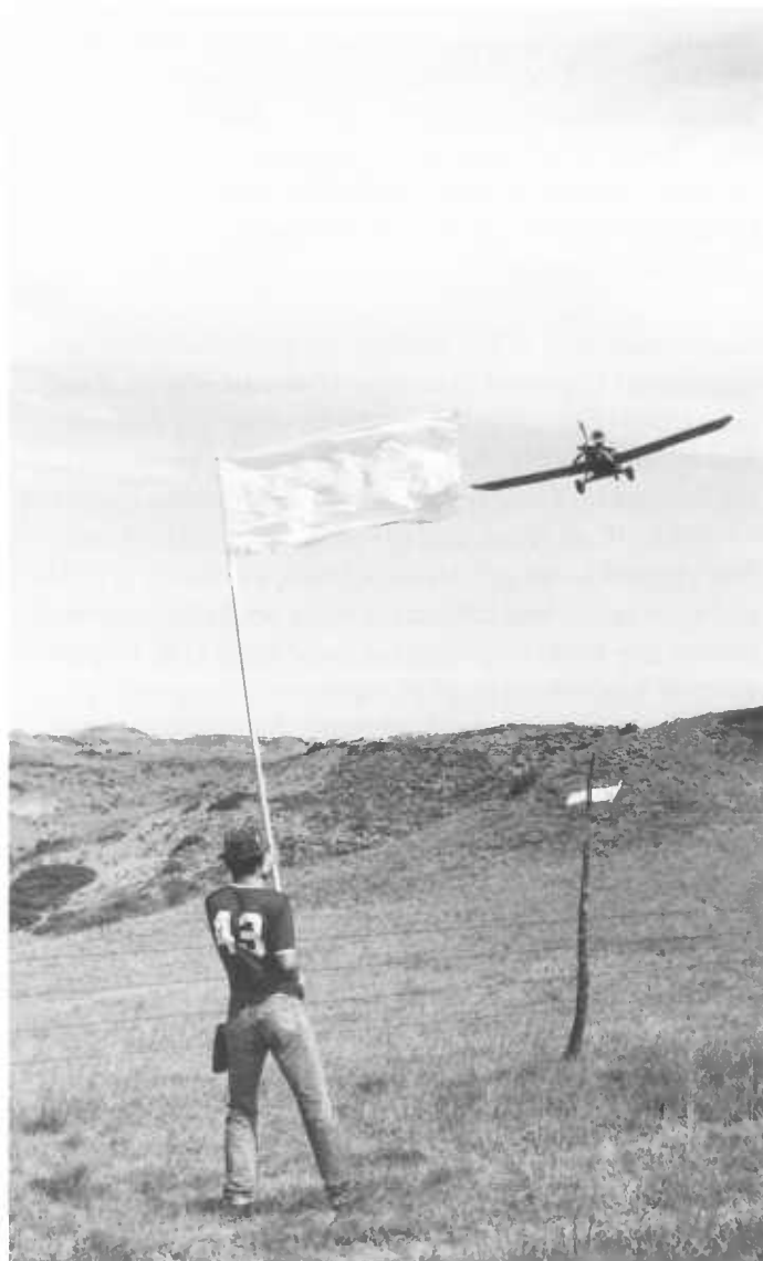
Figure III.8-1 —In the era before global positioning systems, agricultural pilots had to turn the nozzles of their spray equipment on and off manually. Pilots did this when they spotted “flagmen” who stood on the ground at the edge of spray plots or buffer areas. It was virtually impossible to adjust the on/off decision in light of near-ground wind, so insecticide drift was common. Naturally, flagmen were exposed to toxicants just like the target pests! Now, however, computerized equipment on the spray planes can automatically start and stop the flow of pesticides using sophisticated mapping and geostationary satellite coordinates.
