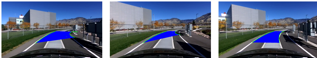
Fig. 6.5: Lane detection frames showing poor detection of lanes or false positives
