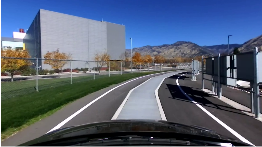
Fig. 4.1: Original image taken on EVR test track. Difficulties for lane detection are shown including shadows, a steep curvature, and shapes similar to lane markers in the center of the road
