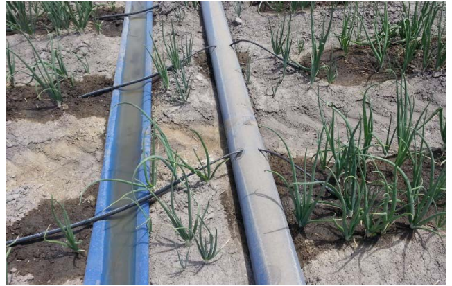
Figure 6. Lay-flat 3-inch manifold connected to 17 mm diameter, 6 mil. wall thickness, drip line.
