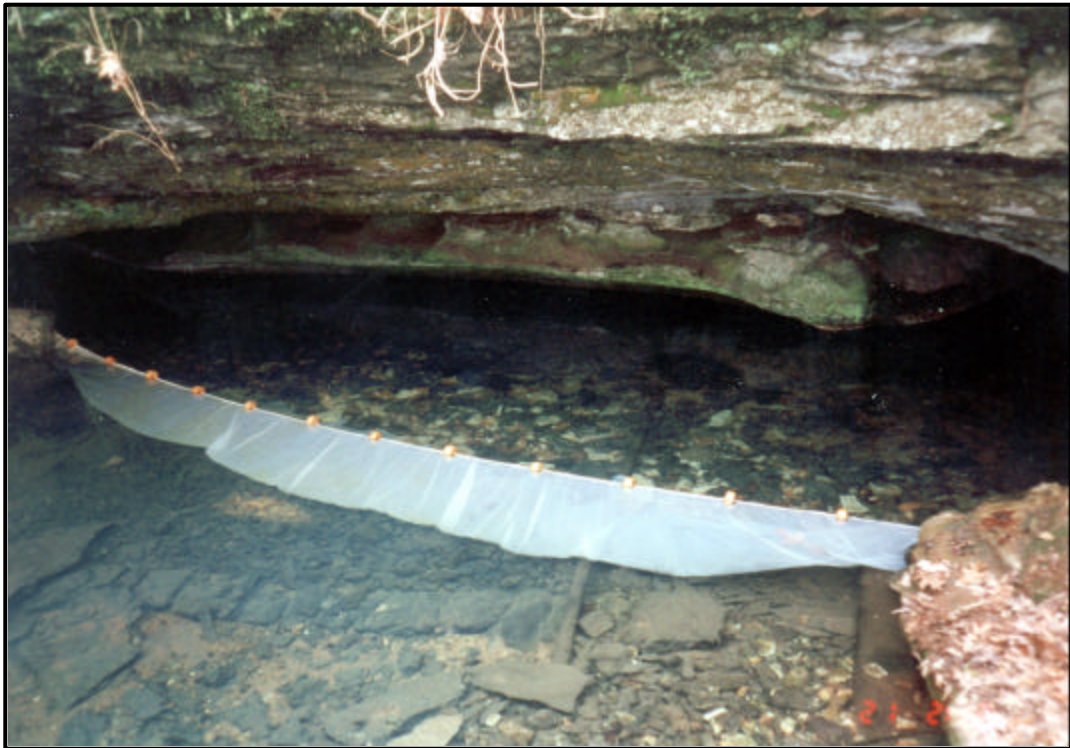
Figure 5. Retention net installed at the mouth of Cave Springs Cave on February 18 th , 2001 with stage = 10.98 ft.
