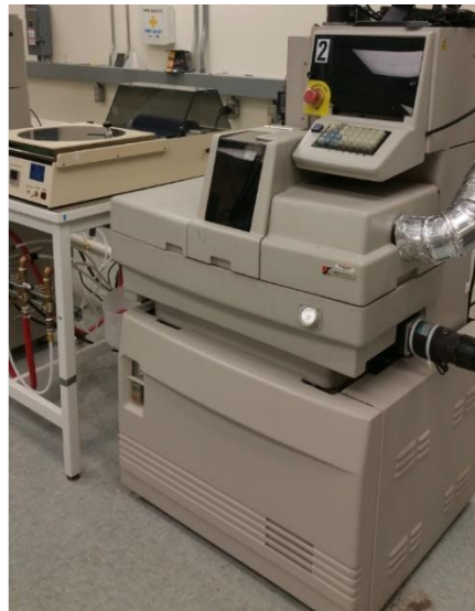
Fig. 5.17. K&S dicing saw used for dicing the DBC substrates
