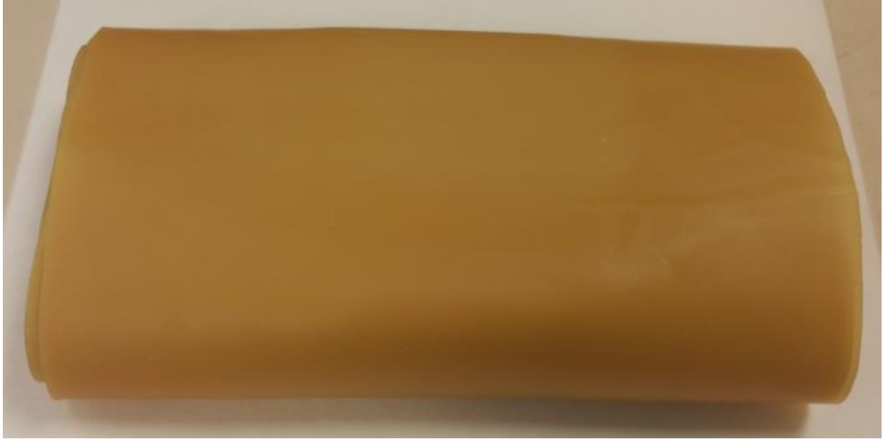
Fig. 5.33. LTCC GreenTape™ assembly wrapped in latex in preparation for lamination
