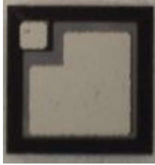
Fig. 5.7. Silicon IGBT device with Ti/Ni/Ag evaporated on the gate and emitter electrodes
