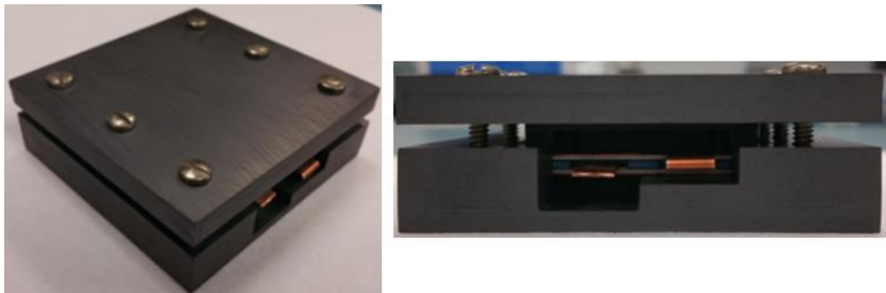
Fig. 5.42. Fixturing used to fabricate the stand-alone power module
