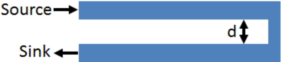
Fig. 2.5. Current conduction loop of an overlapping current path separated by a dielectric
