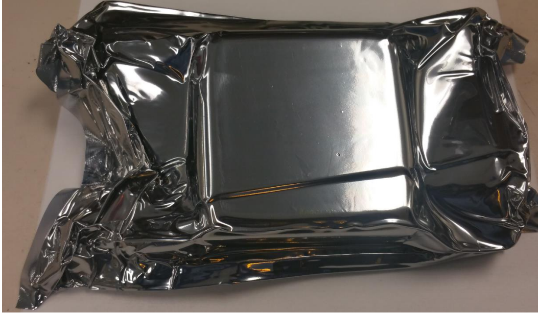
Fig. 5.35. Vacuum sealed LTCC GreenTape™ assembly to carry out lamination process
