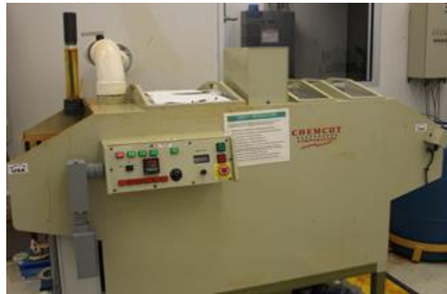
Fig. 5.16. Chemcut spray etcher for chemical etching of DBC
