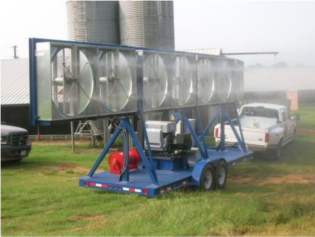
Figure 6. A fan trailer equipped with spray nozzles used for heat mitigation while the trailer is being loaded on the farm. (30.5 to 40.1 °C)
