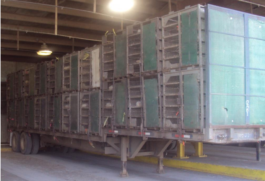
Figure 4. Modules have single side boards for reduced air flow in cool weather conditions.
