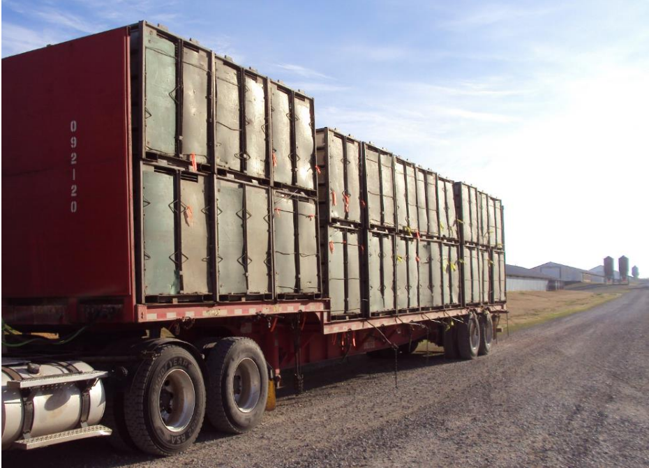
Figure 3. Double side boarded modules for reduced air flow in cold weather.
