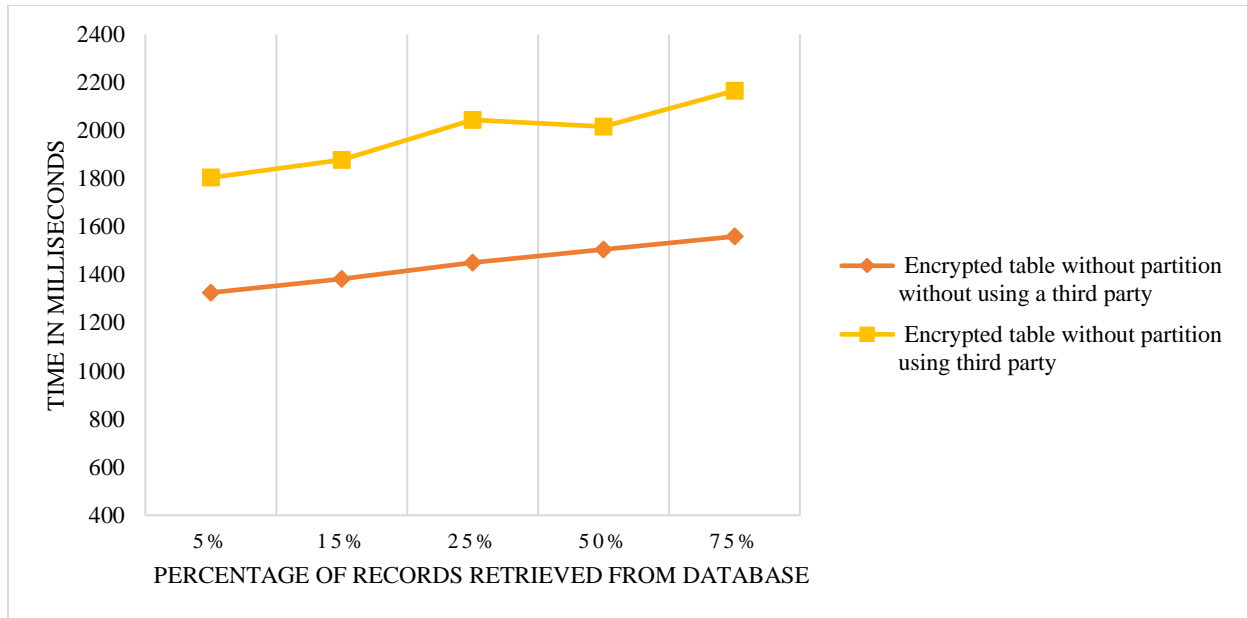
Figure 4.9. Response times for data retrieved from a table having 200,000 records with record size 78 bytes
