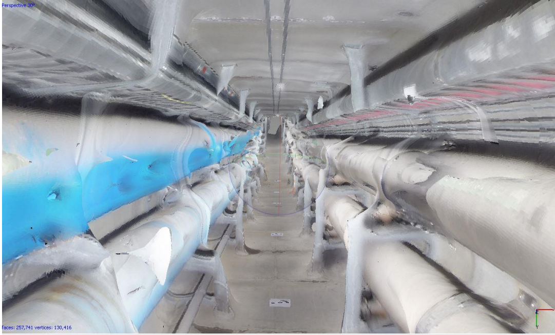
Fig 29. Model generated with individual frames split from continuous GoPro video.
