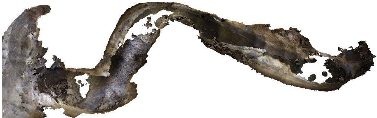
Fig 22. Screen capture of model with ceiling removed to show holes in the floor in areas where there was standing water.
