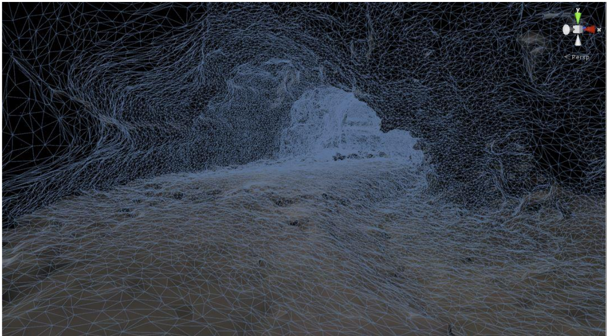
Fig 23. Unity game engine allowed for easy inspection of all parts of the mesh, allowing the user to easily move forwards, backwards, left, right, up, or down, inside the model while simultaneously changing the look direction of the camera.
